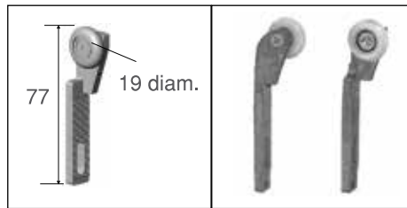
Security/Flyscreen Wheel Assembly S96100 (Pack Set of 2) Max. 10kg each
