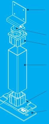
Standard adjustable pier head to support steel or timber bearers
