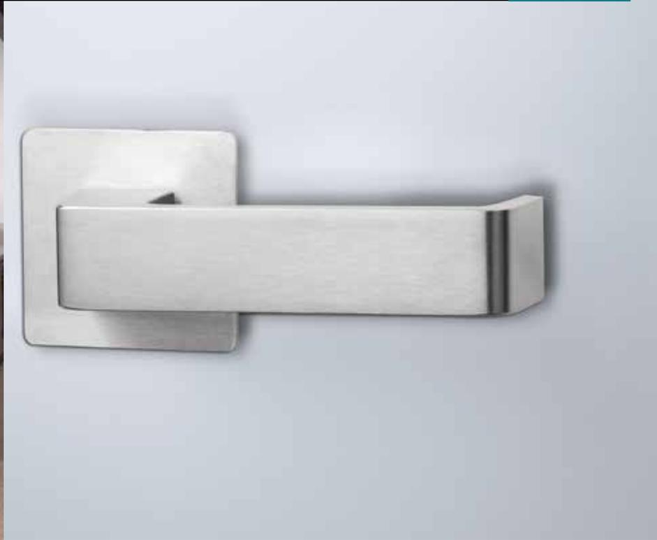
The 260SQ Series door furniture has a 55mm x 2mm square rose. Concealed fixed plates have studs with internal threads located on the rose, visible roses have corresponding countersunk holes and are fixed back to back through the door.
