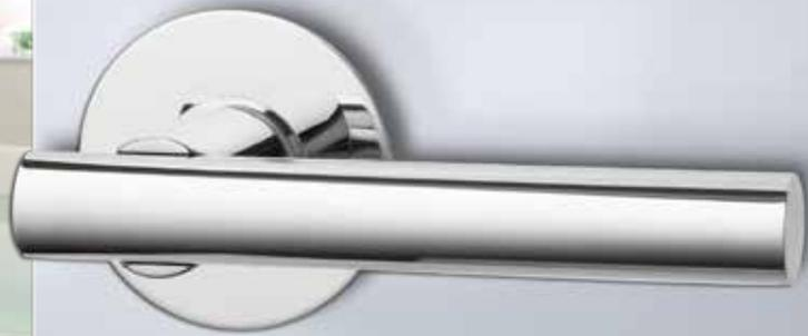
The 260 Series door furniture has a 55mm round rose. Concealed fixed plates have studs with internal threads located on the rose, visible roses have corresponding countersunk holes and are fixed back to back through the door.
