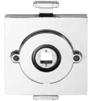
The 3690 Privacy Adaptor has a patented built in clutching mechanism which allows the engaged mode to be overridden by use of specified force applied in a single downward action on the lever. This will allow entry in an emergency situation without the use of any type of tool.
