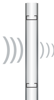
92mm steel studs & 10mm plasterboard on either side.
